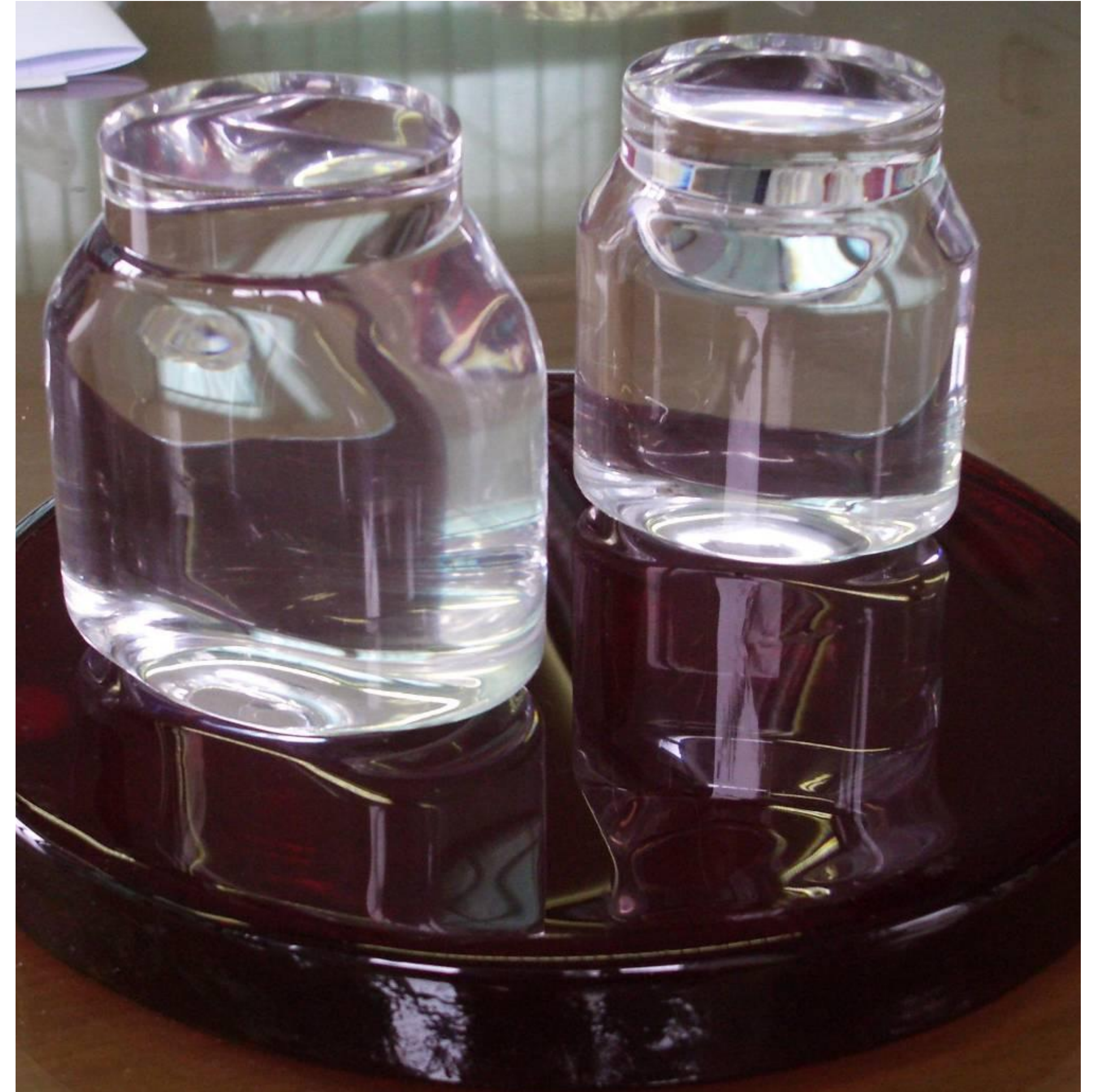
Production of food containers milling from solid and polished
