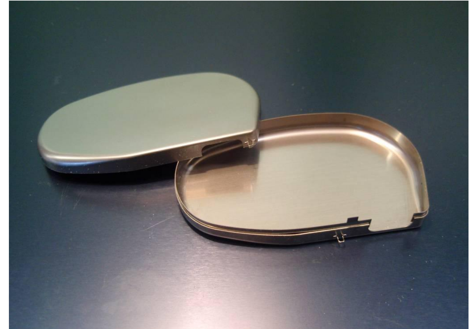
Titanium component processed by cupping, milling and laser micro welding
