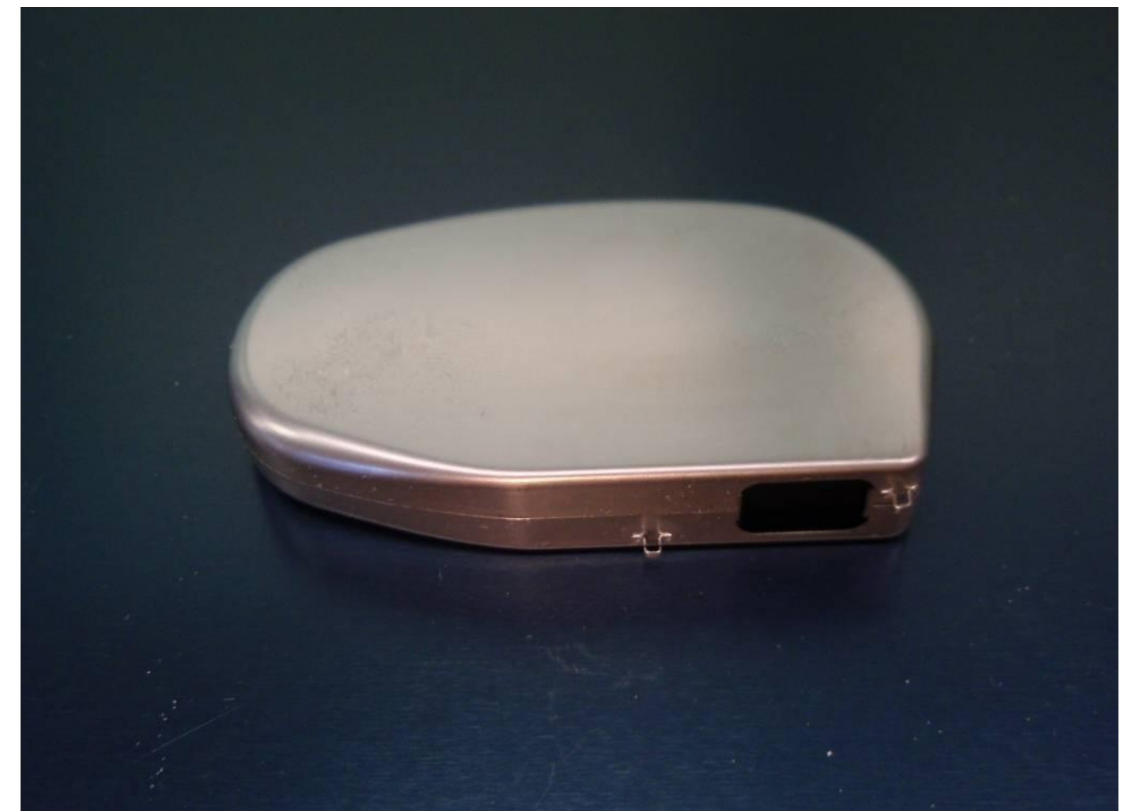
Titanium component processed by cupping, milling and laser micro welding
