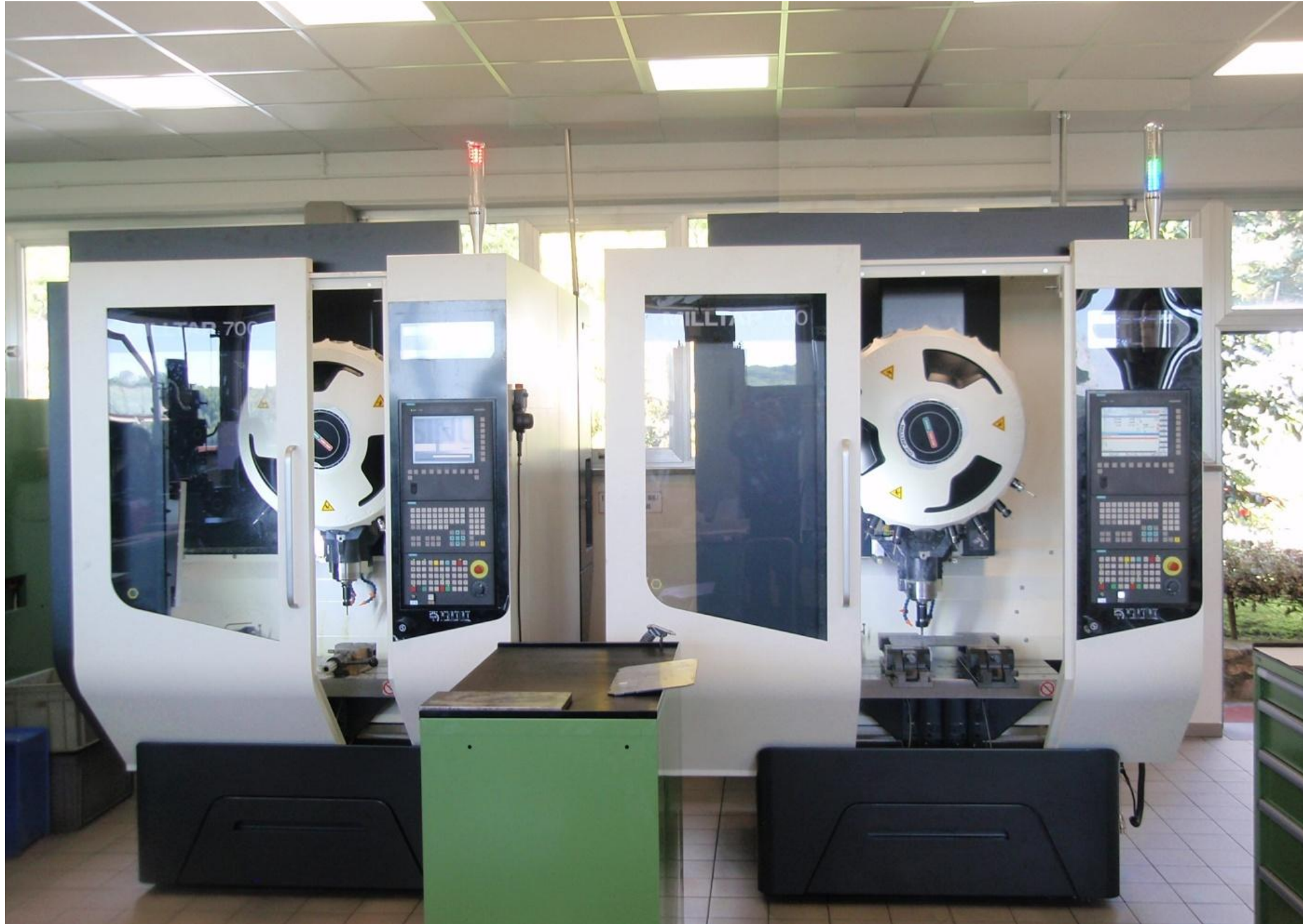
DMG MORI MILLTAP 700 high speed 3 and 5 axle workstation
