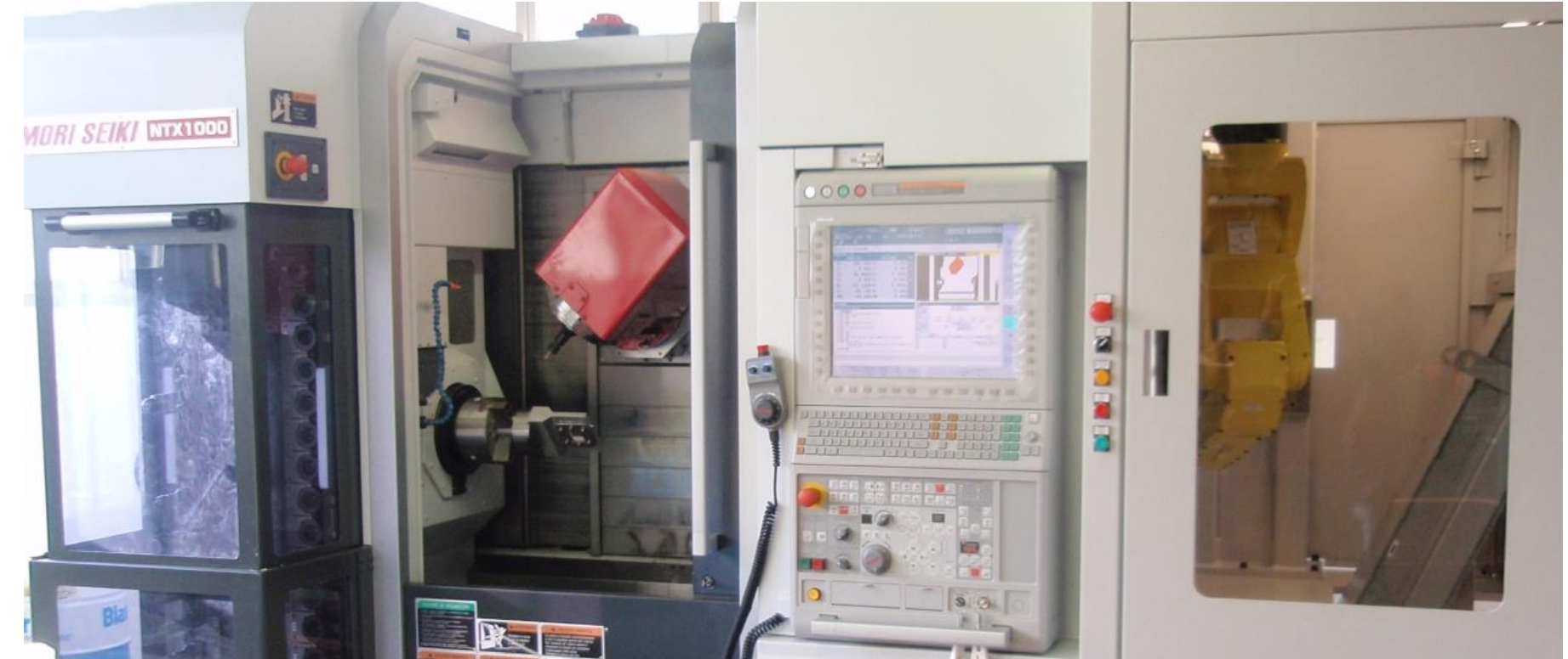
MORI SEIKI NTX 1000 S robotic milling center and 6-axis turning high speed
